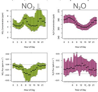
Measurements at the Chamau grassland site show a clear uptake of  $NO_2$  with a pronounced diurnal cycle, and a clear but small  $N_2O$  efflux with a weak diurnal cycle.
