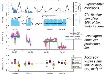
Direct flux measurements of methane with the eddy covariance method are still scarce. The MAIOLICA consortium successfully showed that state-of-the-art flux measurements are able to reproduce a prescribed methane flux with high accuracy (lowest panel). Agreement with prescribed flux is good for both FMA (Fast Methane Analyzer) and QCLAS (Quantum Cascade Laser Absorption Spectrometer) system.
