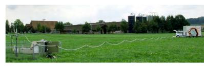
Efforts were made to extend our capability to perform eddy covariance measurements of trace gas fluxes beyond H<sub>2</sub>O, CO<sub>2</sub> and CH<sub>4</sub>. Successful measurements were done with a **Quantum Cascade Laser Absorption Spectrometer** (QCLAS) for N<sub>2</sub>O and NO<sub>2</sub>.
