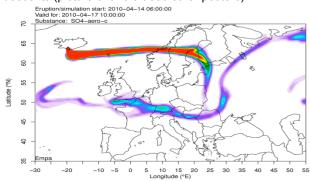
Position of the ash plume (vertically integrated mass) over Europe on 17 April 09:00 UTC simulated by Empa using the model **FLEXPART**
