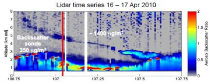
Backscatter ratio measured with the **ETH Aerosol and Cloud Lidar** (Leosphere ALS 450 EZ), 24 h starting from 16 April 18 UTC
